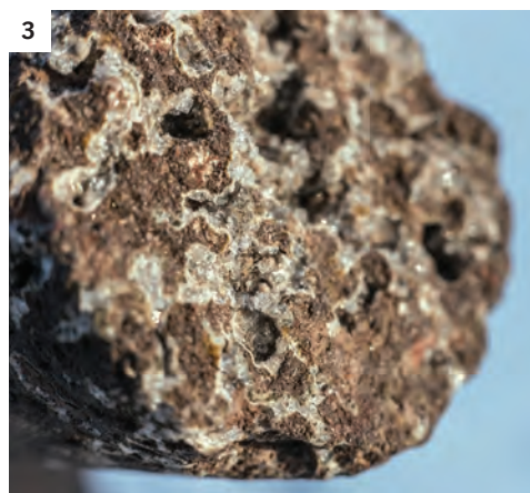
CLIMEWORKS MACHINE extracts carbon dioxide from the atmosphere (1). An injector inside a nearby dome (2) sends the gas more than 700 meters underground, where it reacts with basalt bedrock to form carbonate, visible as white streaks in a core sample from the basalt (3).
